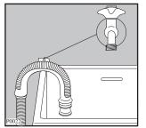
**In a sink drain pipe branch.** This branch must be above the trap so that the bend is at least 60 cm above the ground.
